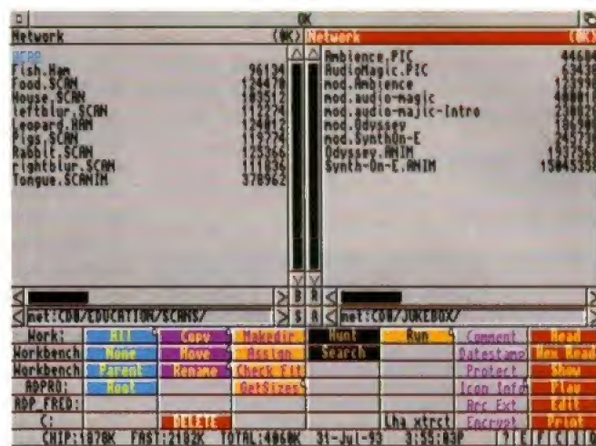
Accessing data from the remote machine using ParBench is just a question of using the device called 'NET:'. This is Directory Opus running on an A3000 accessing Pandora's CD on a CDTV.
